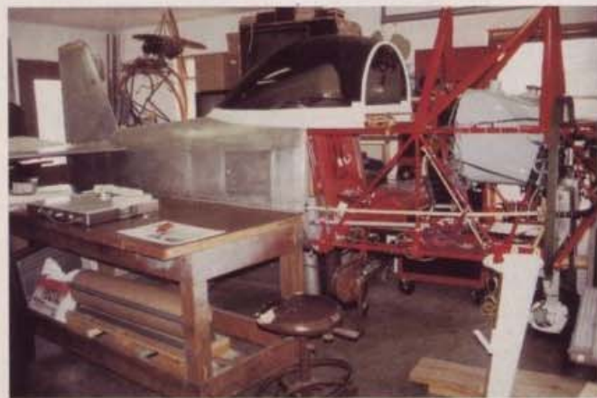
LEFT: Tommy Meyer's Little Toot is seen here undergoing restoration in his father's original workshop. The airplane first flew in 1957. Note the welded steel cockpit truss with semi-monocoque tailcone, with many rivets bucked by a young Tommy Meyer. RIGHT: The Little Toot was redone to match his father's original paint scheme from the 1950s.
