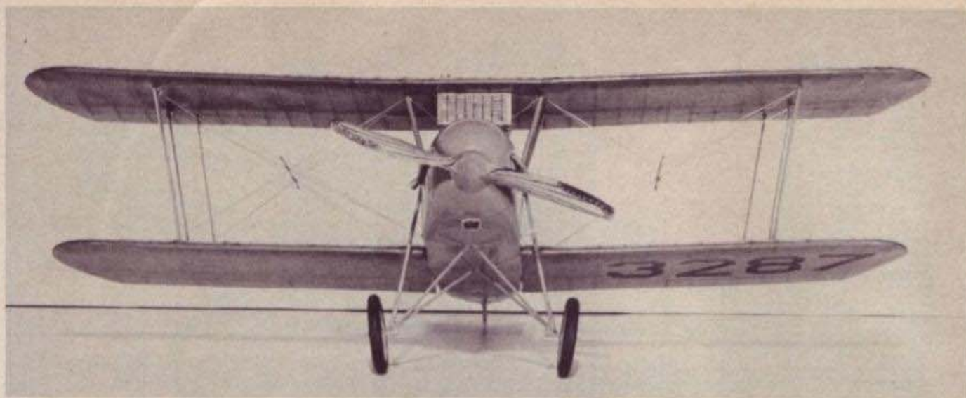
Some changes made at the Waco works. The "Waco 10," straight of panel, in-line mill, OX5 power. It was an able aircraft in its time and age.
